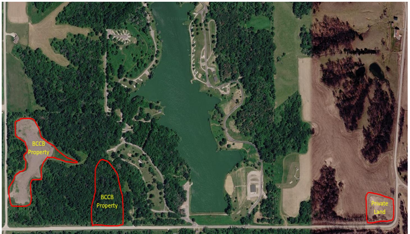
Figure 8. A map highlighting three potential dredge spoil containment sites.
