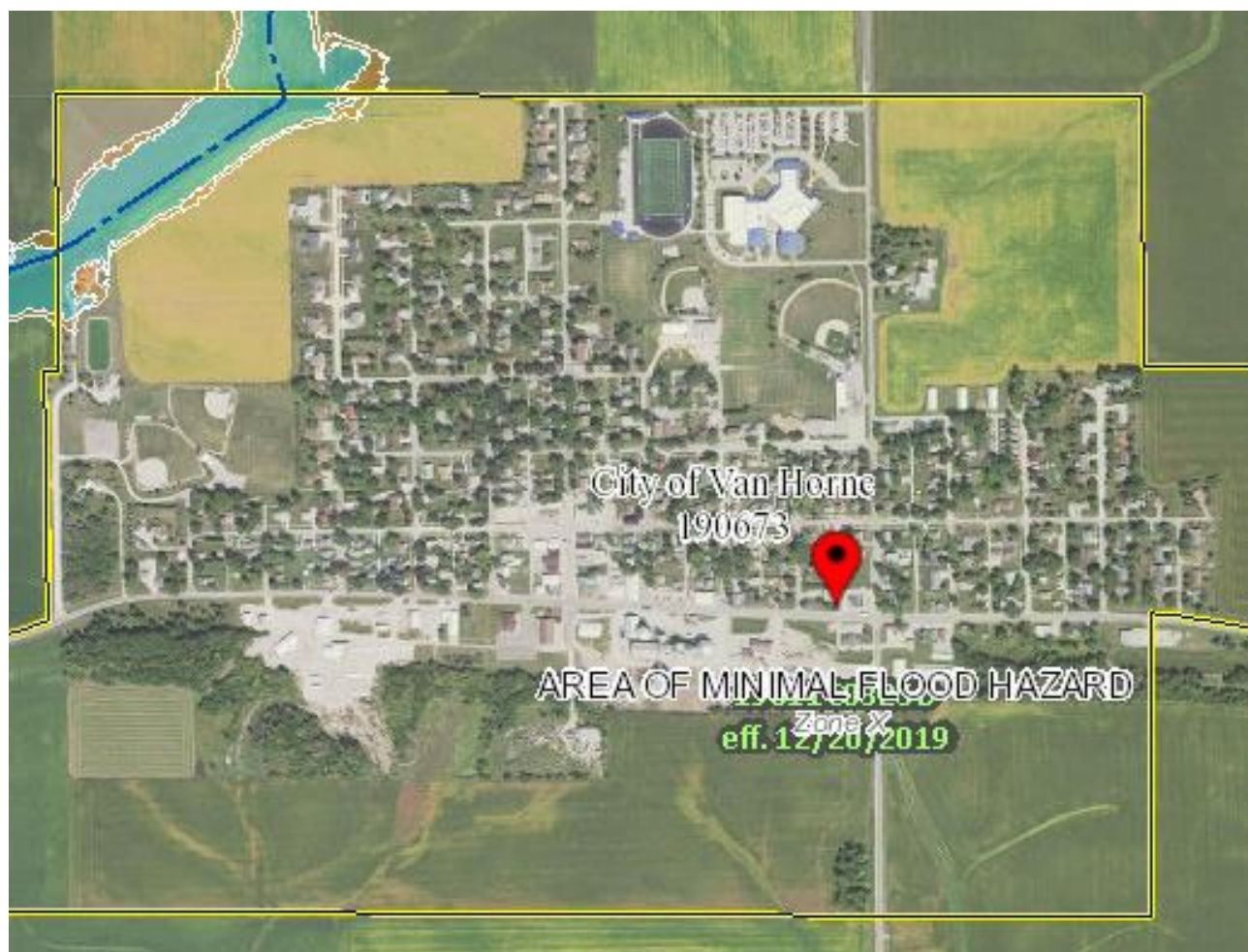
Figure 58: Van Horne 100-Year Flood Hazard Areas
