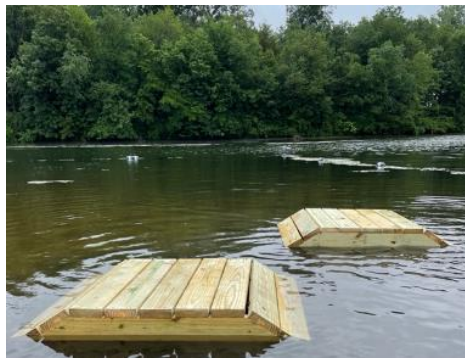
Figure 8: Testing the floatation on two of the three turtle docks in the Rodgers' beach area
